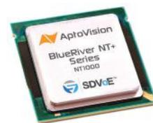
This AV-over-IP chipset lets manufacturers replace traditional AV matrix switches with IP switches to offer a
